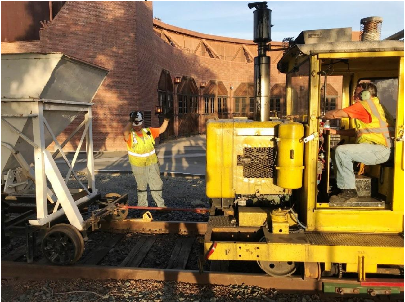
Chris acts as brakeman for Mike H. in the Kalamazoo to remove the skate from under the hopper's wheel
